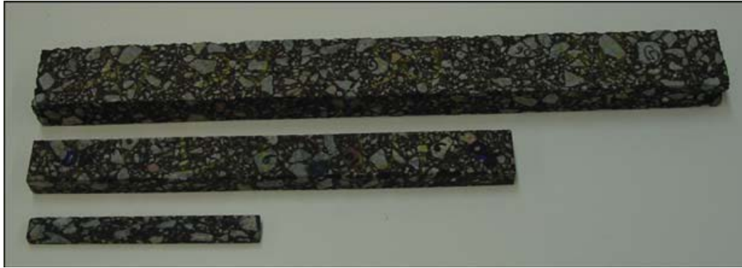
Figure 2.2: 1x, 2x, and 3x asphalt mixture beam specimens. (17)
