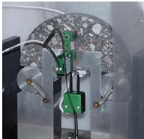
Figure 6.7: The SCB test
