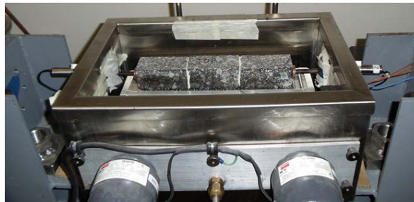
Figure 4.27: Test setup used for the glass transition temperature of beams made from gyratory compacted samples
