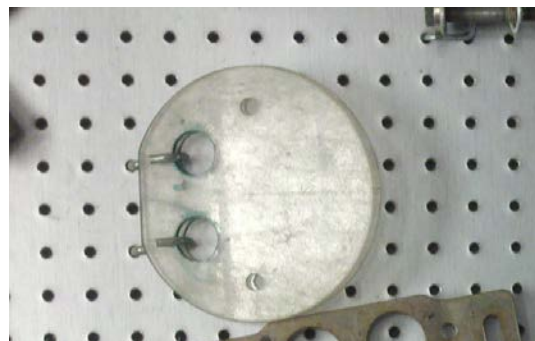
Figure 6.6: DC(T) marking template
