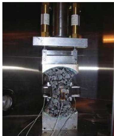
Figure 2.4: Dog-bone direct tension test prototype (27)
