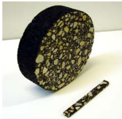
Figure 9.2: IDT and BBR test specimens
